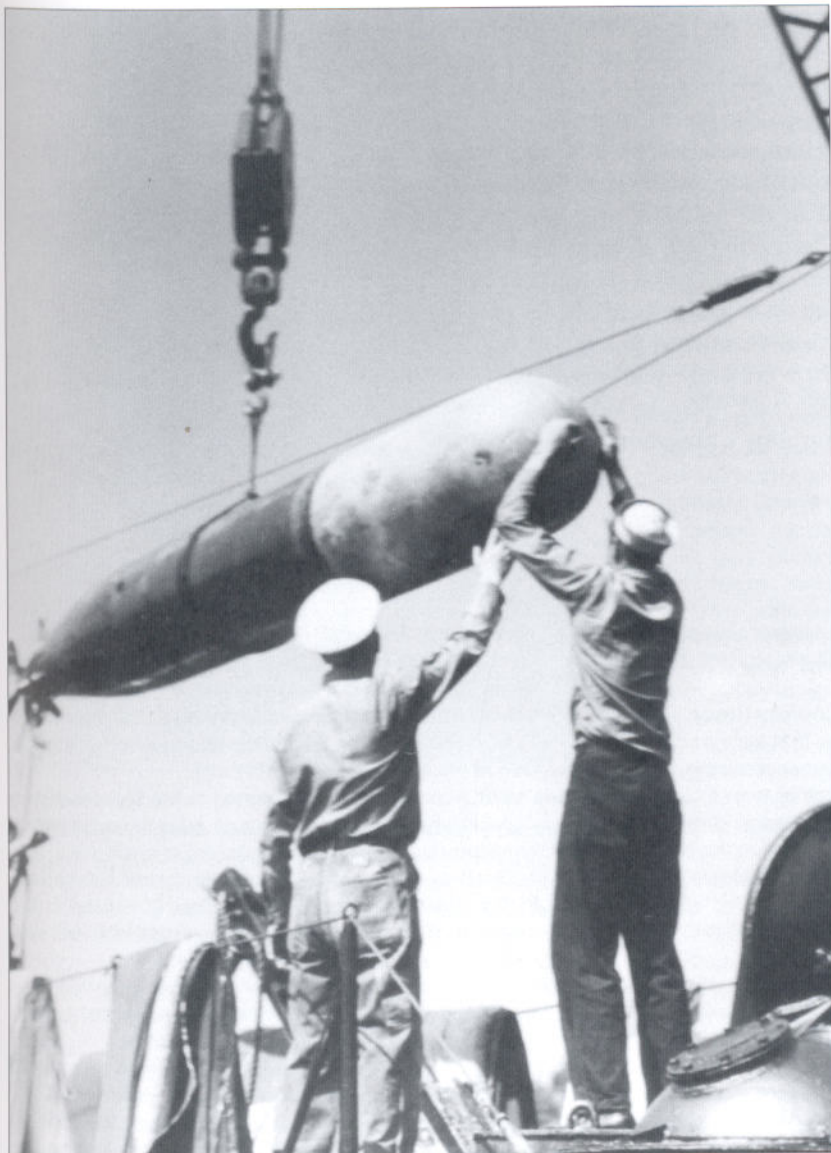
In this 1943 photograph navy personnel load a practice torpedo aboard a submarine at the submarine school at New London. Part of the navy's difficulties in attacks during the War stemmed from lack of extensive practice with the heavier 'war loads' of live torpedoes. (US Navy Photograph)
