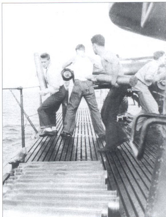
Crew members of a US submarine man the 4-inch/.50-cal. Mk.XII deck gun in this wartime surface drill. By the latter stages of the War US submarines would often engage in surface gun battles with Japanese shipping in order to conserve torpedoes for more difficult targets. (National Archives)
